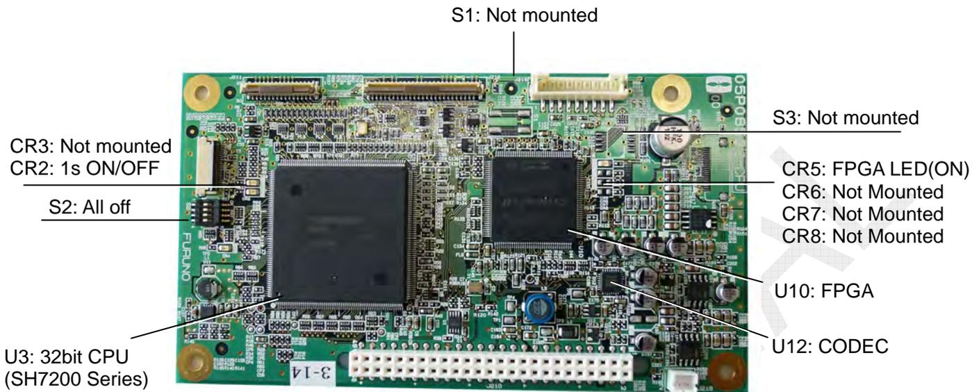
Fig. 2.1.9 C-CPU board: 05P0852 (A-side)
