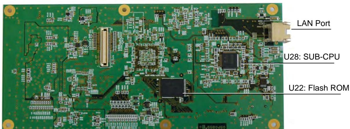
*Fig. 2.5.42 T-CPU board (05P0859) B-side*
