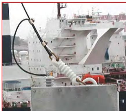
Breaking the connection of lead-in wire may cause burning-out of the Antenna coupler or RT breakdown.
