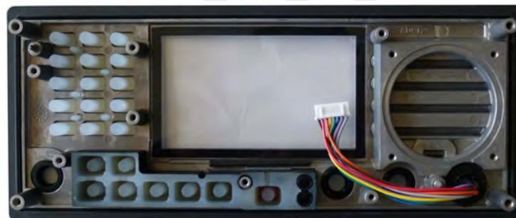
Fig. 2.1.7 Front panel, PANEL board removed
