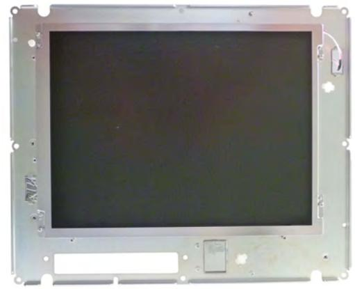
Fig. 2.7.14 Mounting chassis of LCD panel
