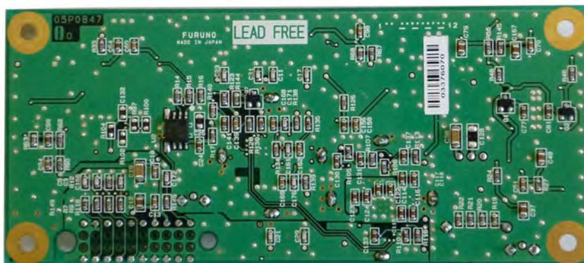
*Fig. 2.5.34 WR1 board (05P0847A) B-side*
