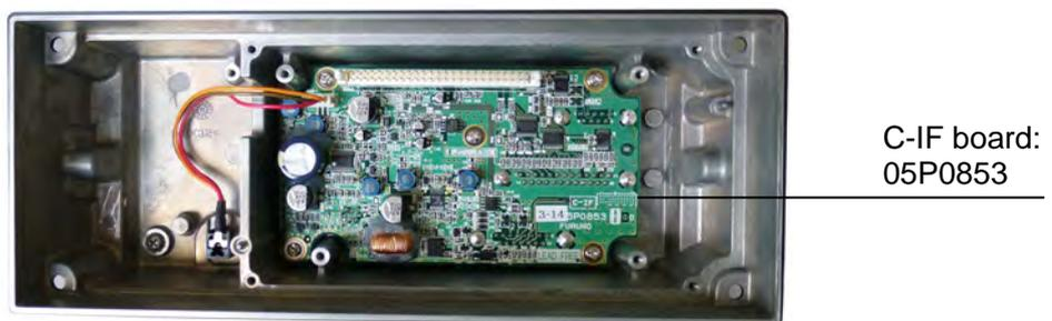
*Fig. 2.1.5 Rear panel, C-CPU board removed*
