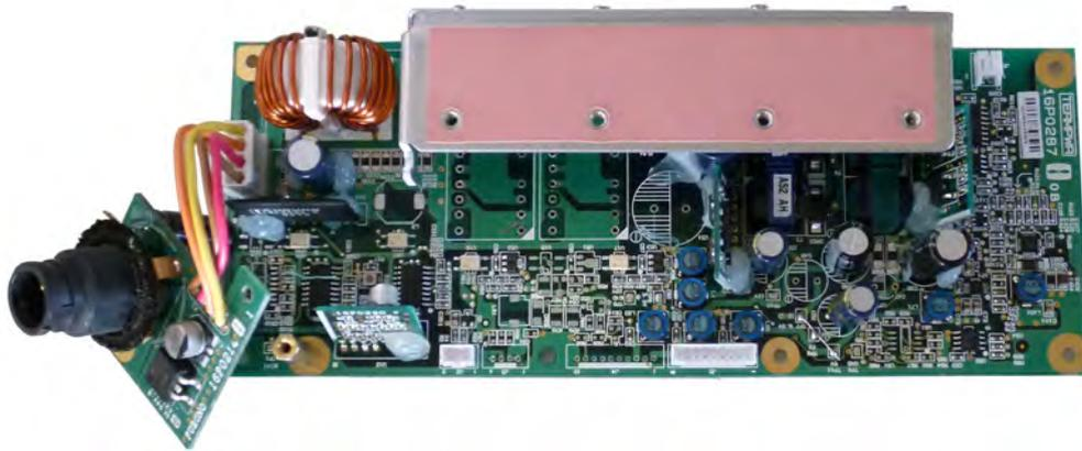
Fig. 2.7.18 TERM PWR board (16P0287A) A-side
